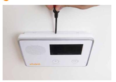
If your panel has a screw on the top, remove it with a crosshead screwdriver so that you can remove the panel cover. To remove the cover, push the two tabs on top and pull the cover out and down. Don't be alarmed if you hear beeping.
