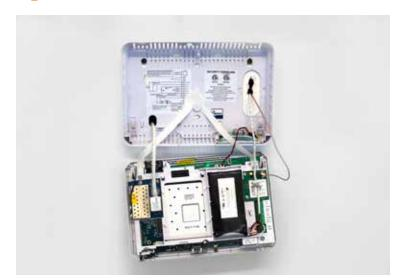
Hang the panel cover on the back plate using the white safety strip.
