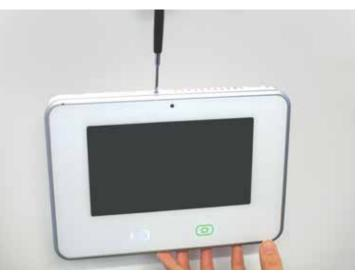
If your panel has a screw on the top, remove it with a crosshead screwdriver so that you can remove the panel
