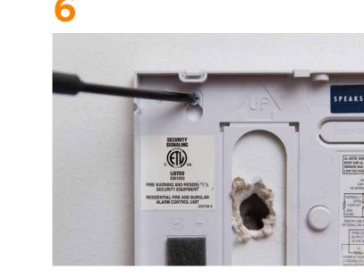
Remove the screws from the backplate of your panel and remove the panel from the wall. Please note there will be a small hole in the wall.
