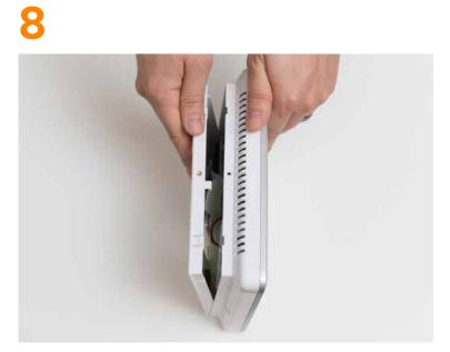
Reassemble your panel by snapping the front cover and backplate together and replacing the top screw.
