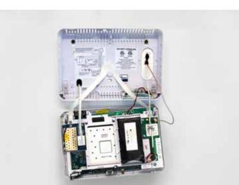
Hang the panel cover on the back plate using the white safety strip.
